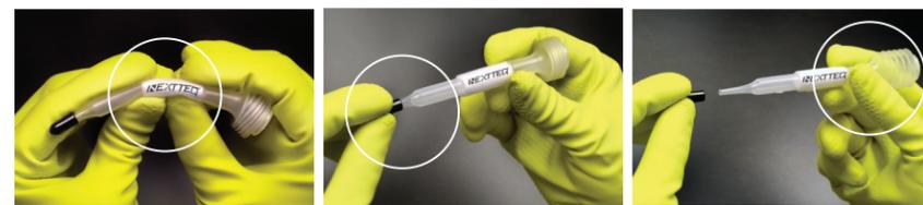
1. Bend smoke generator in the middle to break the ampoule.
