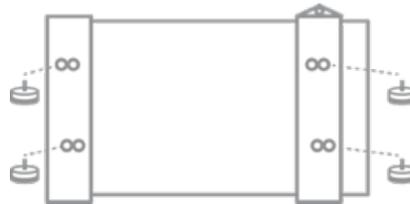
\* NOTE: LEVELING FEET HOLD BRACKET IN PLACE
