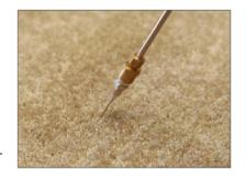
Use of a mild acidic rinse (1 to 320, 1 to 640) like End Zone or Flex Ice will neutralize offensive ammonia salts by lowering pH to the neutral range of 6 to 8 pH. Keep flushing until color of urine or presence of foam is no longer seen through Water Claw<sup>®</sup>. Injection of Bio Release to the pad level after clean-
