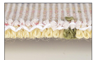
Wilton edge and back view Notice yarns that are not seen as part of the pattern on the face can still be seen in the backing.
