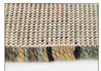
Axminster weave. Note the ribbed appearance of the back and the use of many colors.
