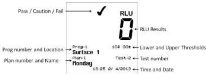
**TIP:** A failed test result **X** can be selected for retesting by pressing the **P** button, followed by the **OK** button to select the Program location (see section [4.2](#)).
