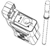
1. Swab the sample area and activate the testing device. (see kit insert for details)
