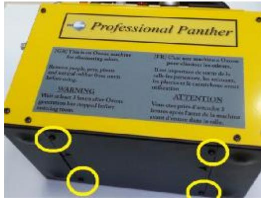
(2) Remove the four (4) screws of the supporting plate at the bottom of the machine.as shown above
