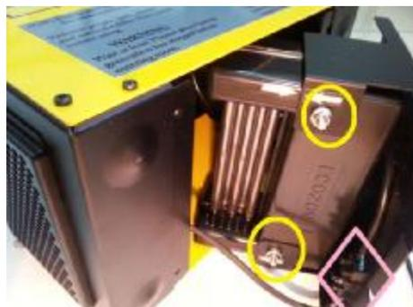
(5) Unscrew the two nuts shown in yellow circles above. This disconnects the Singlet core from its holder. Pull out the screws and gently remove the Singlet core. The result is shown below.
